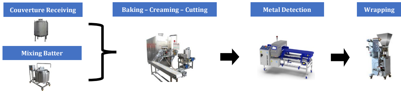
Fig. 6 Flow process of wafer rolls production
