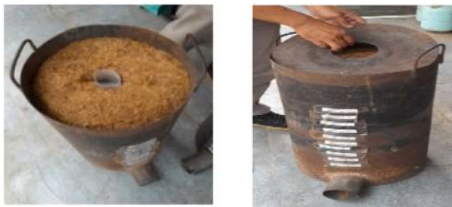
Fig. 3. Bio-stove containing the fine powder of oil palm empty fruit bunches (EFB).
